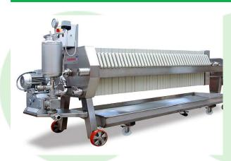
The innovative, new Alpha Magic process is a modern alternative to RDV, for the efficient recovery of valuable juice and wine from material with high solids content.
