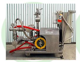
Instead, the juice is pumped into the Velo, pressurized and dosed with a flocculation agent such as bentonite or bentonite/gelatine (gelatine is used for adhering solids and nitrogen used to float the solids).
