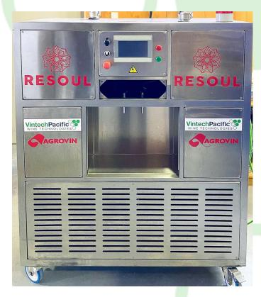
The Resoul system provides a practical and effective method to capture aromatic compounds during alcoholic fermentation and to store and reintroduce those aromas at a later stage, such as at bottling.
